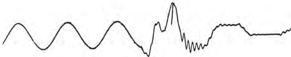
Figure D.3: Field test record of L-G voltage (phase c).
