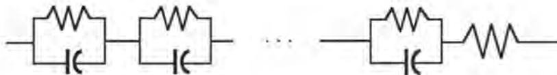
Figure 5.6: A series Foster network used to synthesize a frequency dependent characteristic impedance.
