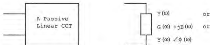
Figure 9.1: The form of the equivalent for a single port network.
